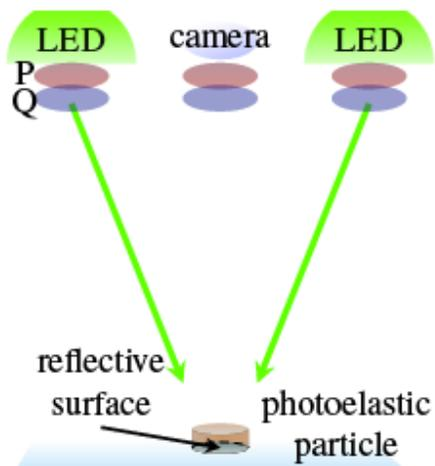
*Using monochromatic light:* Since the stress-optic coefficient of a birefringent materials depends on the wavelength of light, it is best to record monochromatic light for quantitative results. There are two main ways to do this. (1) Use colored LED lights. (2) Filter the light reaching the camera. This could be either a screw-on filter that attaches to the camera lens (possibly in series with the polarizer), or by just analyzing one RGB channel of a full-color image.
