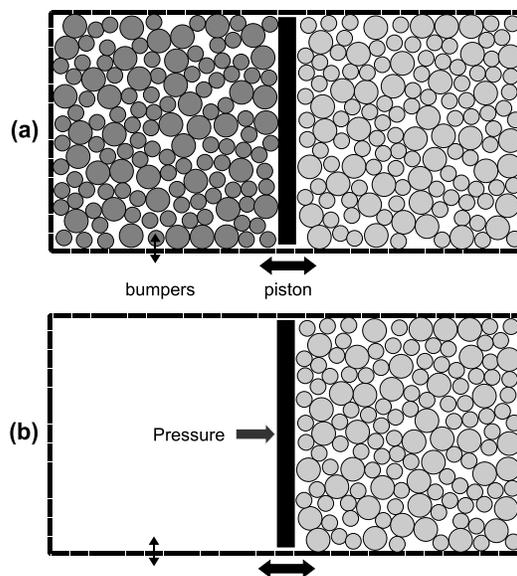
**FIGURE 1.** Schematic of the apparatus used to measure the dynamics under (a) volume equilibration (b) and constant pressure conditions. In the volume-equilibration case, an equal number of particles with different properties are placed in “thermal” contact and allowed to equilibrate under agitation from the sidewalls. In the constant-pressure (or constant-volume, not shown) case, the properties of a single set of particles are examined.
