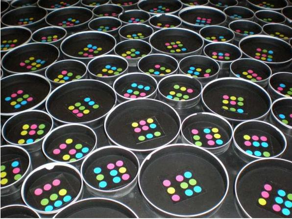
**FIGURE 2.** Photograph of large and small particles, showing unique identifier patterns.
