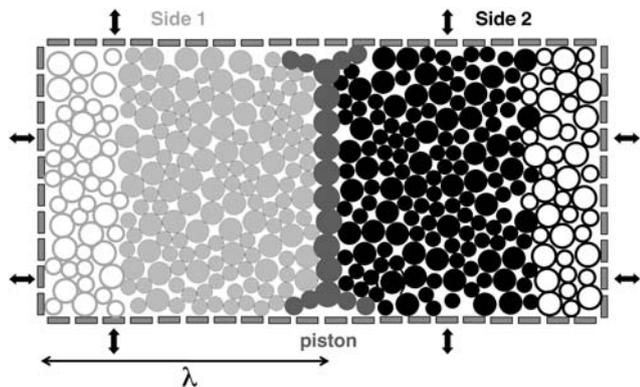
**Fig. 1** Apparatus schematic (1 m  $\times$  2 m), with particles drawn to scale. Filled particles are taken from an experimental configuration and indicate the size of the imaged region.  $\lambda$  between 0 and 1 measures the fractional position of the piston.
