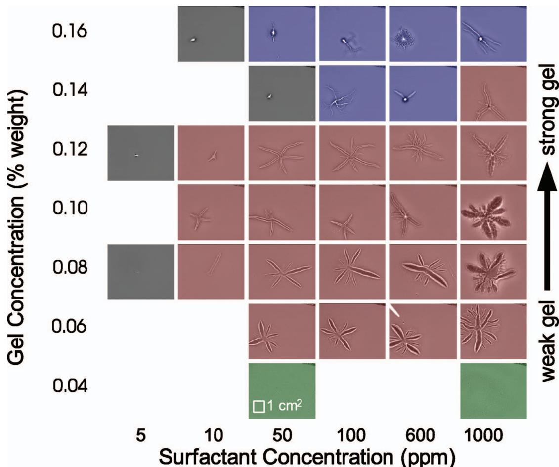
FIG. 1. Phase diagram for droplets of nonionic surfactant solution (Triton X-305) spreading on a viscoelastic agar gel substrate. Red images: starburst instability; blue images: wispy drops; green images: uniform spreading.
