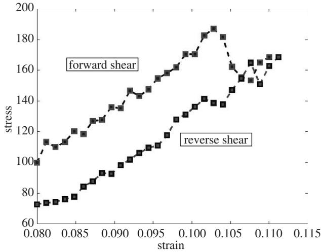
Figure 6. Mean pressure in the biaxial experiment as a function of shear strain,  $\epsilon = \Delta L/L$ . The system is deformed from  $\epsilon = 0$  to a value slightly greater than 0.11, and then cycled back to a net strain of  $\epsilon = 0.08$ . Note the stress drops at local failure events, and the overall stress drop after the system has been returned to  $\epsilon = 0.08$ .
