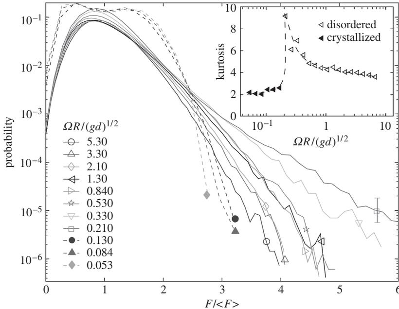
Figure 9. Probability distributions for the force, measured at the bottom of the layer for the indicated shear rates,  $\Omega$ . Two-peaked distributions pertain to the ordered state, and single-peaked distributions to the disordered state. The tail of the distributions stretches out at the transition point. This feature leads to cusps in various moments for the force distribution, such as the kurtosis, which is given in the inset.
